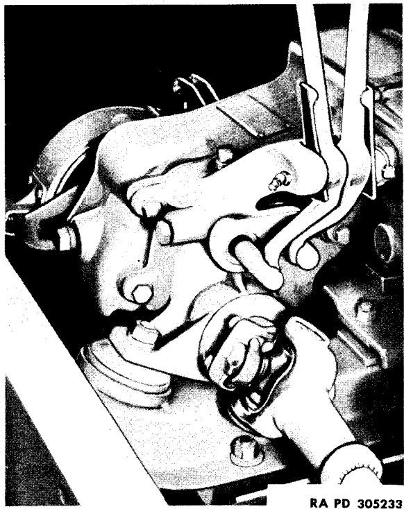
Figure 73—Transfer Case Shifting Mechanism
