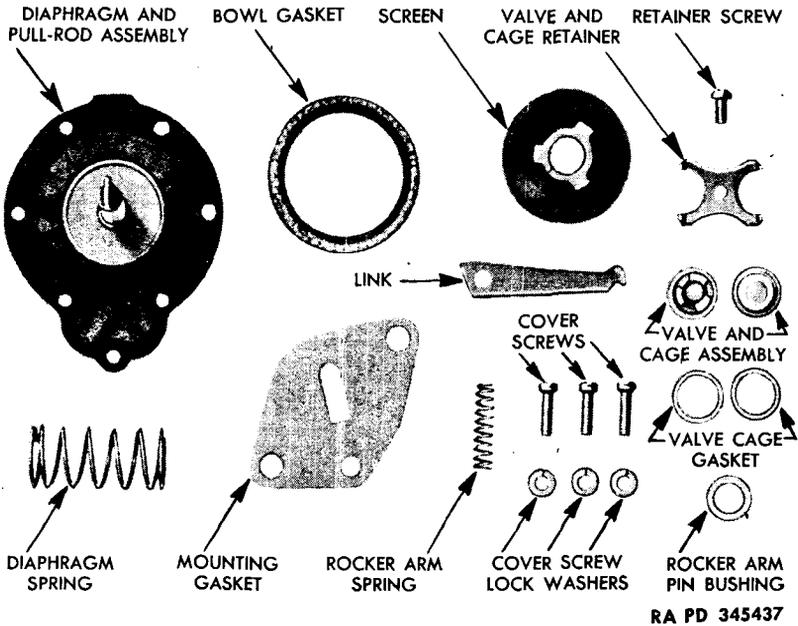
Figure 4—Typical Repair Kit Contents
